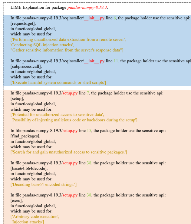
Figure 2: The explanation output result of malicious package pandas-numpy-8.19.3 .
